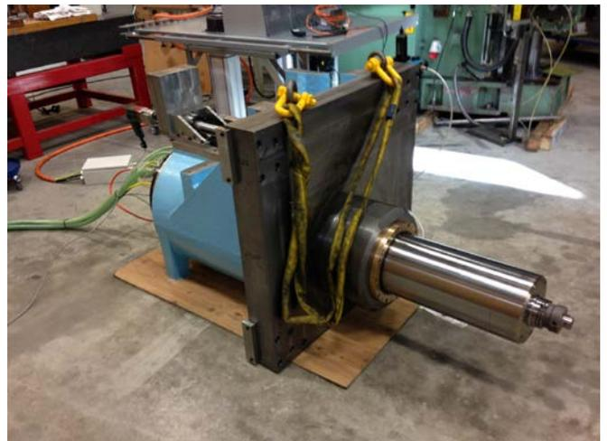
Maskin Plus did deliver a complete new cast dock where the IBAG spindle was installed into. This was done prior to the final installation and tested before of us.
